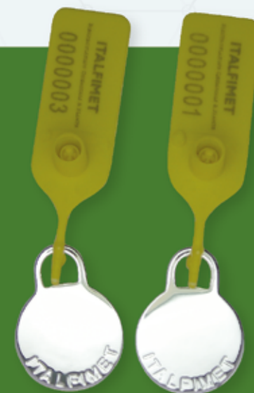
SAMPLES PRE AND POST TREATMENT COLORIMETRIC COORDINATES: PRE TREATMENT OBJECT L=99.0 a=0 b=3.2 POST TREATMENT OBJECT L=98.6 a=0 b=3.8
