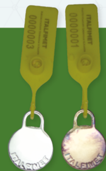
SAMPLES AFTER OXIDATION TEST: PASSIVATED SAMPE (LEFT) NOT PASSIVATED SAMPLE (RIGHT) *SOLUTION OF AMMONIUM SULPHUR 2%
